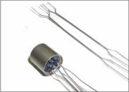
Fine welding of electronic components, e.g., thermocouples
