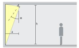
Wallwashing For uniform vertical illuminance, the distance (a) of Optec lens wallwashers from the wall should be around one third of the room height (h). This results in an angle of tilt ( $\alpha$ ) of approx. 35°.
