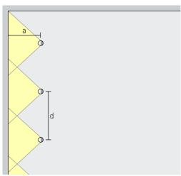
For good longitudinal uniformity, the luminaire spacing (d) of Optec wallwashers may be up to 1.2 times the distance to the wall (a).
