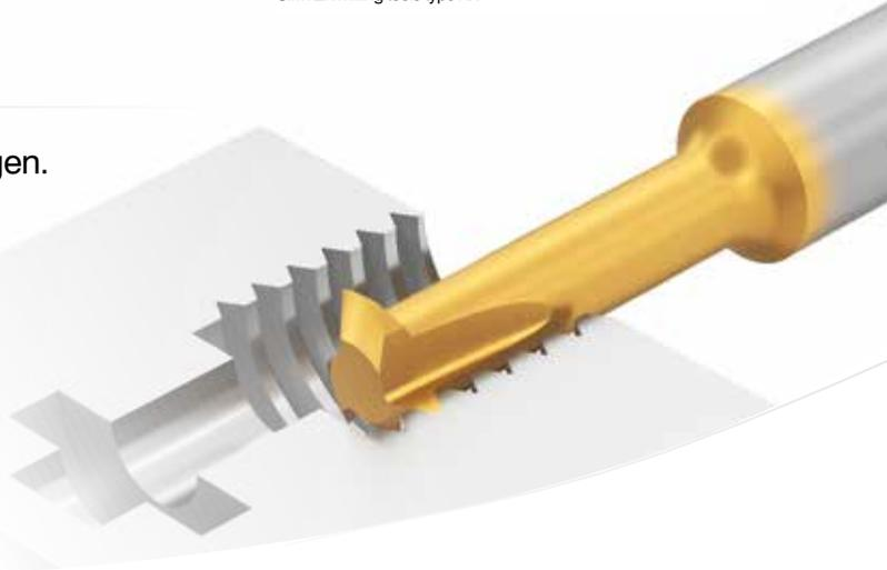
Solid micro grain carbide milling cutter for groove milling applications in bores as of min.  $\varnothing$  1,4 mm. Available with three and partly with four edges. High groove depths as well as extended thread depths at low cutting pressure are possible with this system.
